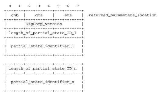
Figure 13: Format of returned SigComp parameters
