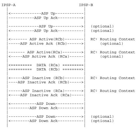
In this approach, only one single exchange of ASP Up message can be considered as enough since the response by the other peer can be considered as a notice that it is in ASP\_UP state.
