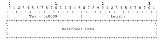
The Heartbeat Data parameter contents are defined by the sending node. The Heartbeat Data could include, for example, a Heartbeat Sequence Number and/or Timestamp. The receiver of a BEAT message does not process this field as it is only of significance to the sender. The receiver MUST respond with a BEAT Ack message.
