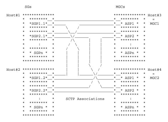
SGP1.1 and SGP1.2 are part of SG1 SGP2.1 and SGP2.2 are part of SG2
