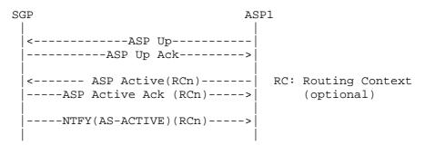
Note: If the ASP Active message contains an optional Routing Context parameter, the ASP Active message only applies for the specified RC value(s). For an unknown RC value, the SGP responds with an Error message.
