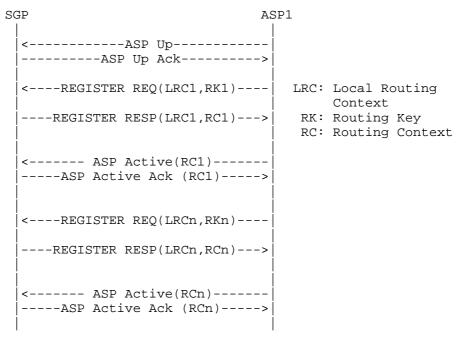
Note: In the case of an unsuccessful registration attempt (e.g., invalid RKn), the Register Response message will contain an unsuccessful indication and the ASP will not subsequently send an ASP Active message. Each LRC/RK pair registration is considered independently.
