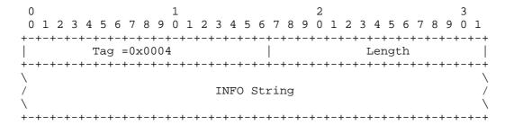
The format and description of the optional INFO String parameter is the same as for the DUNA message (See Section 3.4.1). The INFO String in an ASP Up Ack message is independent from the INFO String in the ASP Up message (i.e., it does not have to echo back the INFO String received).
