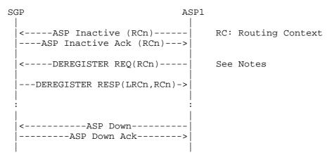
Note: The Deregistration procedure will typically be used if the ASP previously used the Registration procedures for configuration within the Application Server. ASP Inactive and Deregister messages exchanges may contain multiple Routing Contexts.
