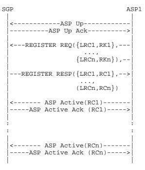
Note: In the case of an unsuccessful registration attempt (e.g., Invalid RKn), the Register Response message will contain an unsuccessful indication and the ASP will not subsequently send an ASP Active message. Each LRC/RK pair registration is considered independently.
