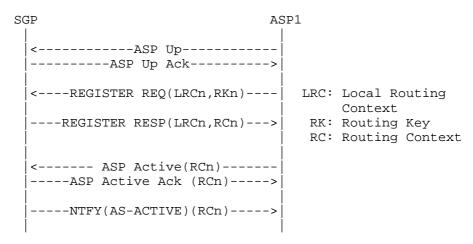
Note: In the case of an unsuccessful registration attempt (e.g., invalid RKn), the Register Response message will contain an unsuccessful indication and the ASP will not subsequently send an ASP Active message.
