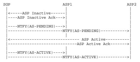
Note: If the SGP M3UA layer detects the loss of the M3UA peer (e.g., M3UA heartbeat loss or detection of SCTP failure), the initial ASP Inactive message exchange (i.e., SGP to ASP1) would not occur.
