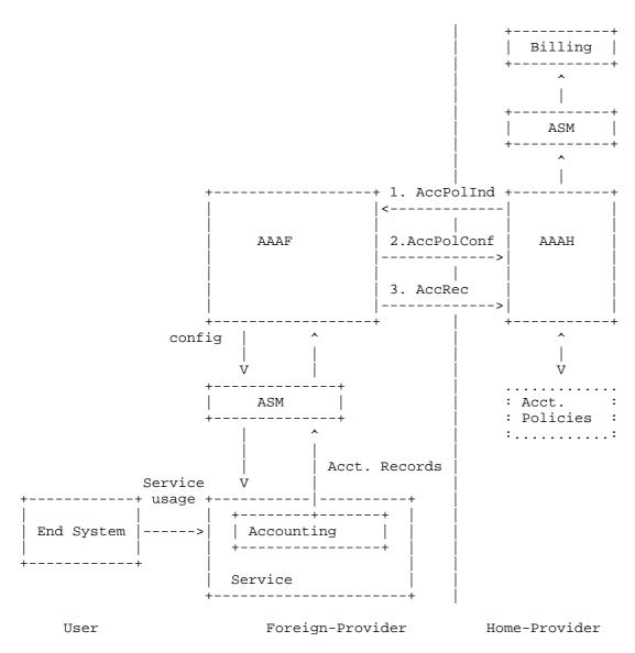
Figure 8: Inter-Domain Accounting (Roaming Example)
