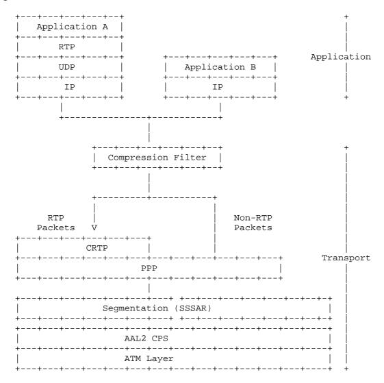
In the picture above, application A is an RTP application generating RTP packets. Application B is an IP application generating IP datagrams. Application A gathers the RTP data and formats an RTP packet. Lower level layers of application A add UDP and IP headers to form a complete IP packet. Application B is generating datagrams to the IP layer. These datagrams may not have UDP or RTP headers.
