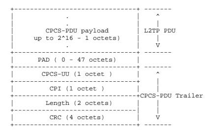
The Common Part Convergence Sub-layer (CPCS) PDU payload field contains user information up to  $2^16 - 1$  octets.
