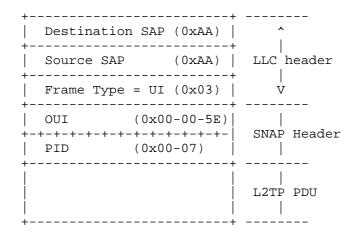
Note: The format of the overall AAL5 CPCS PDU is shown in the next section.
