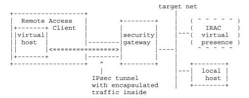
In this case, the IRAC system begins with an externally routable address. An additional target network address is assigned to the IRAC, and packets containing this assigned address are encapsulated, with the outer headers containing the IRAC's routable address, and forwarded to the IRAS through the tunnel. This provides the IRAC with a virtual presence on the target network via an IPsec tunnel. Note that the IRAC now has two active addresses: the ISP-assigned address, and the VIP.
