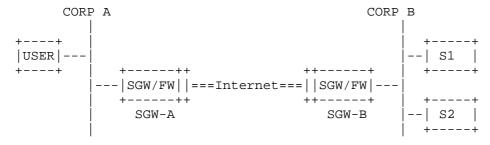
This is purposely simplified in order to illustrate some basic characteristics without getting bogged down in details. At the edge of each network is a combination security gateway and firewall device. These are labeled "SGW-A" and "SGW-B". In this diagram, corporation B wishes to provide a user from corporation A with access to servers S1 and/or S2. This may be accomplished in one of several different ways:
