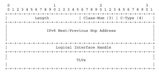
See [RFC2205] for a description of hop address and handle fields. See [RFC3471] for a description of parameters and encoding of TLVs.
