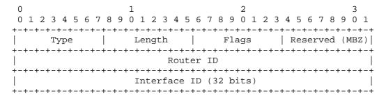
The Type is 4 (Unnumbered Interface ID); the Length is 12. Flags are defined below.
