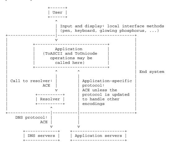
The box labeled "Application" is where the application splits a domain name into labels, sets the appropriate flags, and performs the ToASCII and ToUnicode operations. This is described in section 4.
