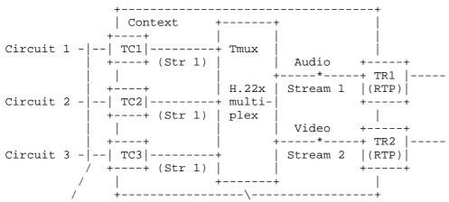
Figure 6: Multiplexed Termination Scenario - Single to Multiple
