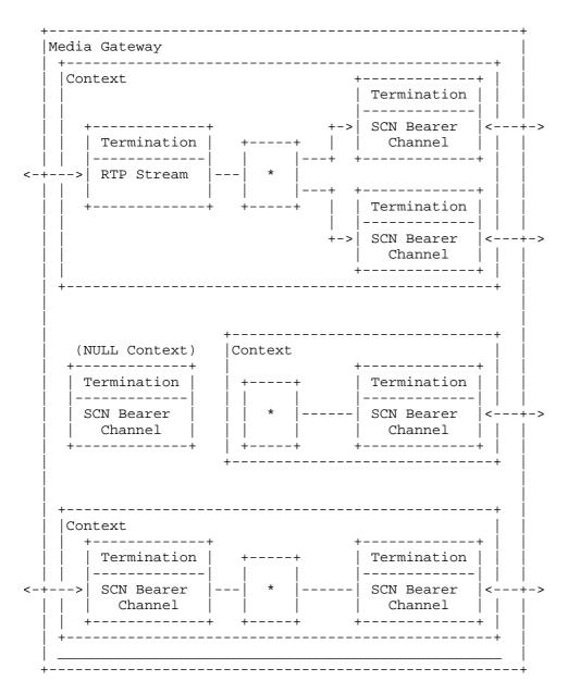
Figure 1: Examples of Megaco/H.248 Connection Model
