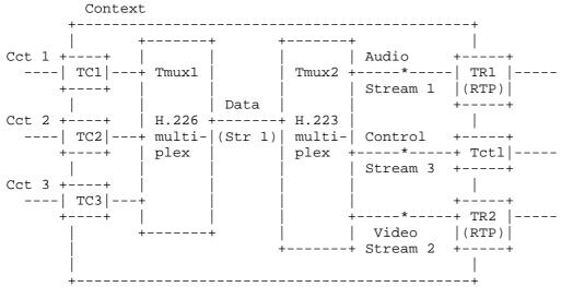
Tmux1 has a Multiplex Descriptor and a single data stream. Tmux2 has a Multiplex Descriptor with a single bearer and three explicit Stream Descriptors.
