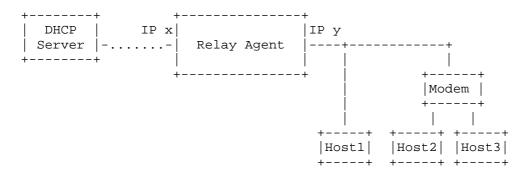
In the usual approach, the relay agent would put IP address Y into the giaddr of any packets that it forwarded to the DHCP server. However, if for any reason, IP address Y is not accessible from the DHCP server, this approach will fail. There are several reasons why IP y might be inaccessible from the DHCP server:
