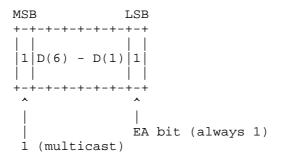
Figure 2. Address mapping in multicasting (MAPOS version 1).
