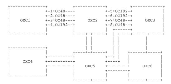
Figure 6: Mesh Optical Network with SRLGs
