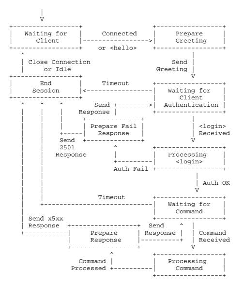
Figure 1: EPP Server State Machine
