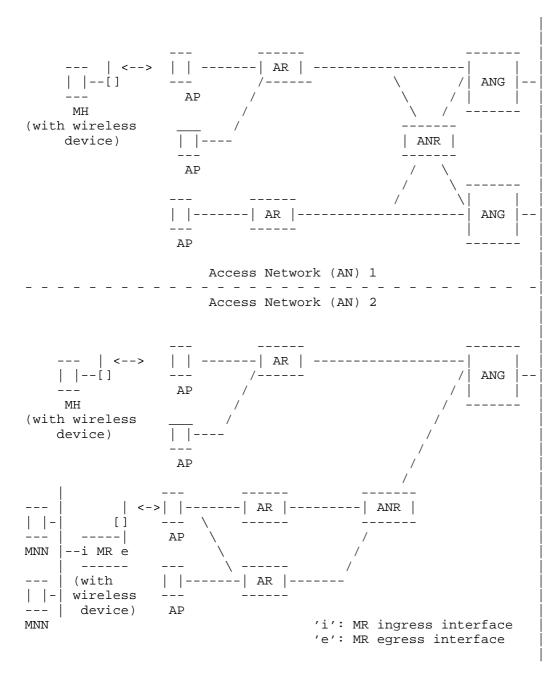
Figure 1: Reference Network Architecture
