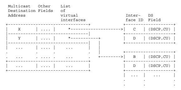
Figure 8: Multicast routing table with additional fields for DSCP values
