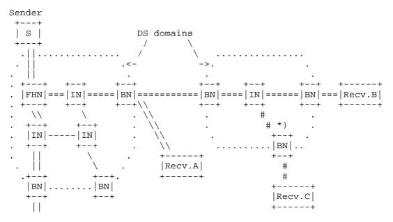
FHN: First-Hop Node, BN: Boundary Node, Recv.x: Receiver x
