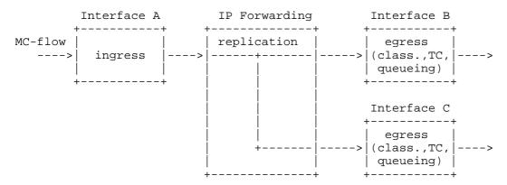
Figure 1: Multicast packet replication in a DS node
