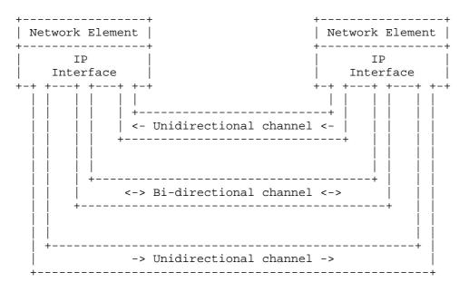
As mentioned above, a typical example of a multi-channel link is a cellular wireless link. In this example, header compression would be applicable on a per-channel basis, for each channel operating either in a bi-directional or unidirectional manner, depending on the channel properties.
