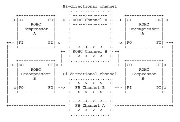
In this example, feedback is, in both directions, sent on its own dedicated channel, as discussed in e.g., feedback realization example 1-3 of ROHC [RFC-3095, page 44]. With this configuration, the piggybacking/interspersing mechanism of ROHC is not used, and the PI/PO connections are thus left open (marked with a "o"). It should
