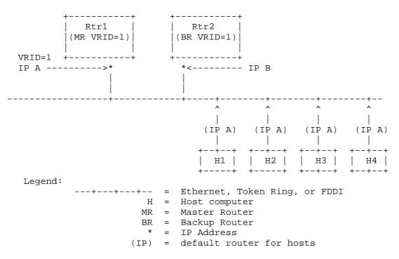
Eliminating all mention of VRRP (VRID=1) from the figure above leaves it as a typical IP deployment. Each router is permanently assigned an IP address on the LAN interface (Rtr1 is assigned IP A and Rtr2 is assigned IP B), and each host installs a static default route through one of the routers (in this example they all use Rtr1's IP A).
