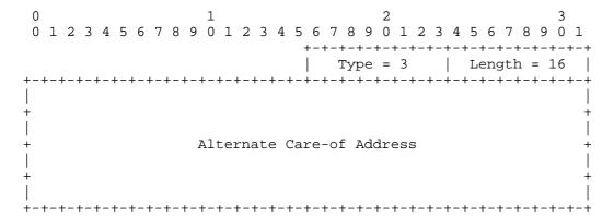
Normally, a Binding Update specifies the desired care-of address in the Source Address field of the IPv6 header. However, this is not possible in some cases, such as when the mobile node wishes to indicate a care-of address which it cannot use as a topologically correct source address (Section 6.1.7 and Section 11.7.2) or when the used security mechanism does not protect the IPv6 header (Section 11.7.1).
