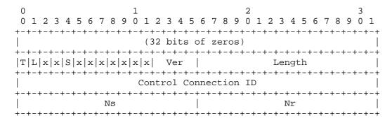
Named fields are as defined in Section 3.2.1. Note that the Length field is still calculated from the beginning of the control message header, beginning with the T bit. It does NOT include the "(32 bits of zeros)" depicted above.
