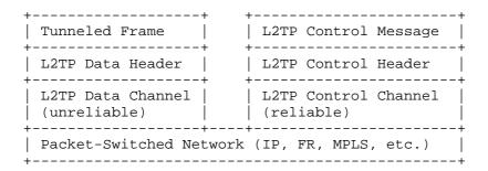
Figure 3.0 depicts the relationship of control messages and data messages over the L2TP control and data channels, respectively. Data messages are passed over an unreliable data channel, encapsulated by an L2TP header, and sent over a Packet-Switched Network (PSN) such as IP, UDP, Frame Relay, ATM, MPLS, etc. Control messages are sent over a reliable L2TP control channel, which operates over the same PSN.
