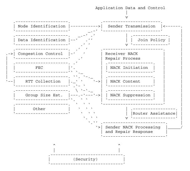
Fig. 1 - NORM Building Block Framework
