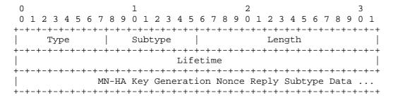
Figure 5: The Generalized Mobile IP MN-HA Key Generation Nonce Reply Extension
