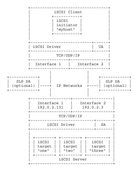
In the above drawing, the iSCSI server has three iSCSI targets that the client could discover, named "one", "two" and "three". The iSCSI client has an iSCSI initiator with the name "myhost". The iSCSI client may use the initiator name in its SLP Service Requests as a filter to discover only targets that are configured to accept iSCSI connections from "myhost".
