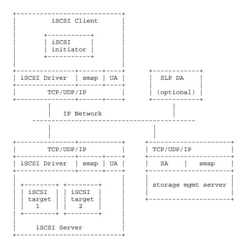
Note the difference between the storage management server model and the previously defined target discovery model. When target discovery was used, the iSCSI Server implemented an SA, to be discovered by the initiator's UA. In the storage management server model, the iSCSI clients and servers both implement UAs, and the management server implements the SA.
