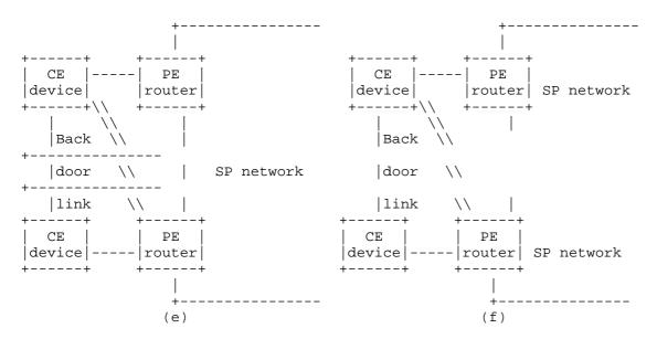
Figure 2.1. Representative types of access arrangements
