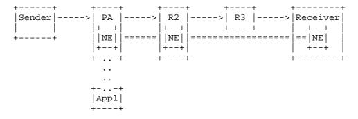
Appl = signaling PA = Proxy for signaling application application
