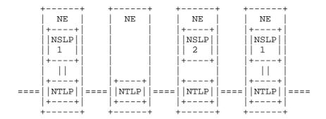
Figure 5: Signaling with Heterogeneous NSLPs
