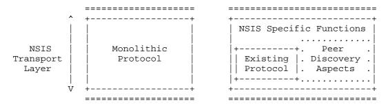
Figure 6: Options for NTLP Structure
