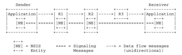
Figure 1: Simple Signaling and Data Flows
