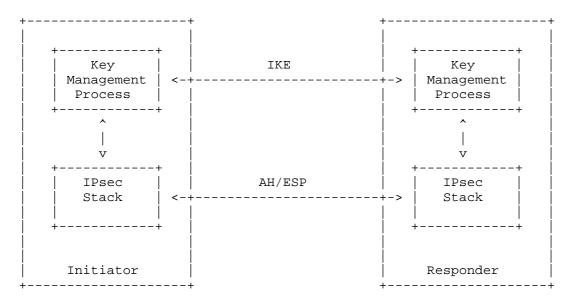
The general deployment model for IKE is shown above. The IPsec engines and IKE engines typically are separate modules. When no security association exists for a packet that needs to be processed (either sent or received), the IPsec engine contacts the IKE engine and asks it to establish an appropriate SA. The IKE engine contacts the appropriate peer and uses IKE to establish the SA. Once the IKE handshake is finished it registers the SA with the IPsec engine.
