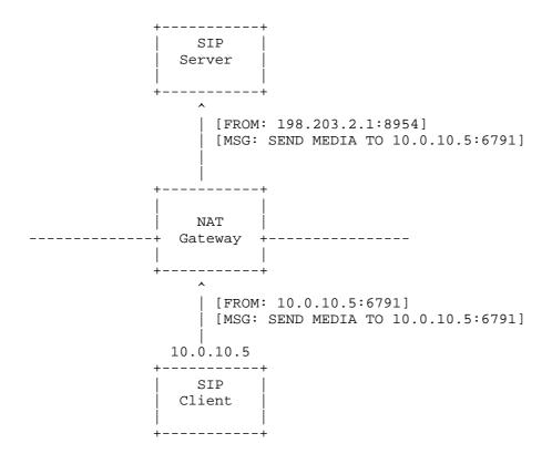
The purpose of STUN is to allow clients to detect this situation and determine the address mapping. They can then place the appropriate address in their application-level messages. This is done by using an external STUN server. That server is able to determine the translated address and tell the STUN client, as shown below.
