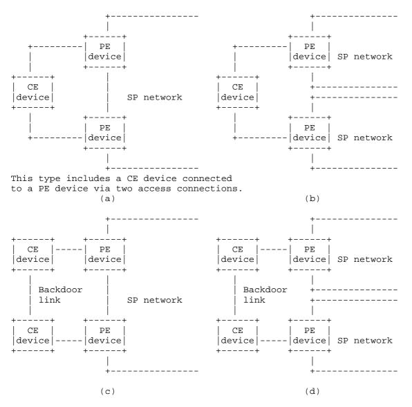
Figure 2.4: Four types of double-homing arrangements.
