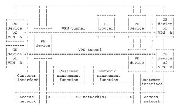
Figure 2.7: Reference model for layer 3 provider-provisioned CE-based VPN.
