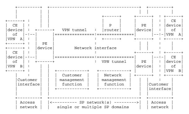
Figure 2.1: Reference model for layer 3 PE-based VPN.
