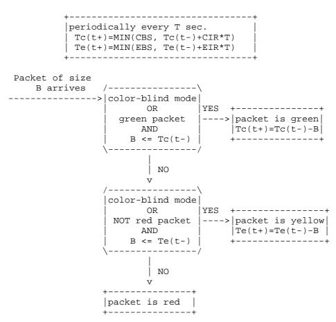
Figure 1: Traffic Metering/Marking Algorithm
