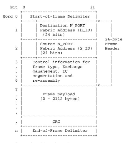
Figure 4. Fibre Channel Frame Format
