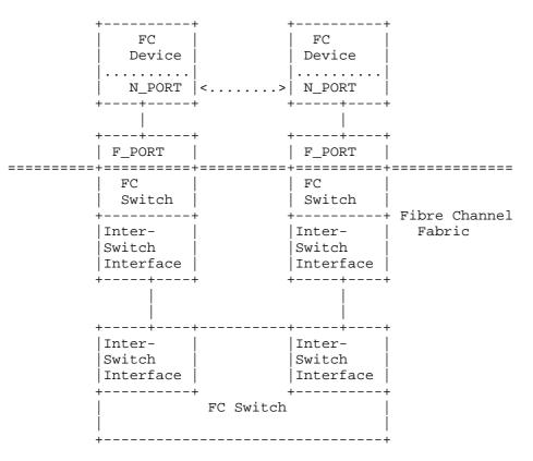
Figure 2. Multi-Switch Fibre Channel Fabric
