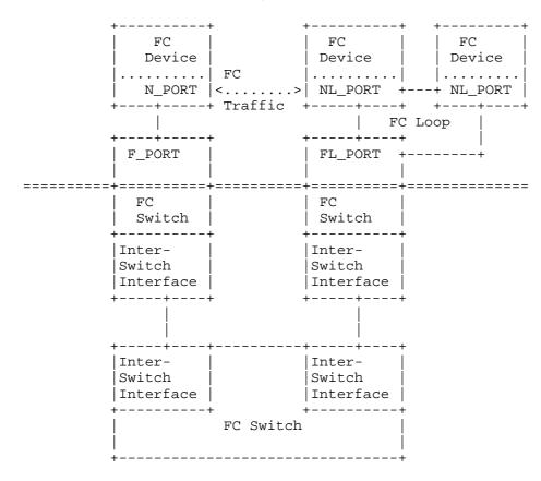
Figure 3. Mixed Fibre Channel Fabric
