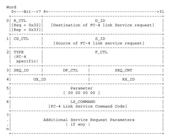
Figure 19. Format of an FC-4 Link Service Frame
