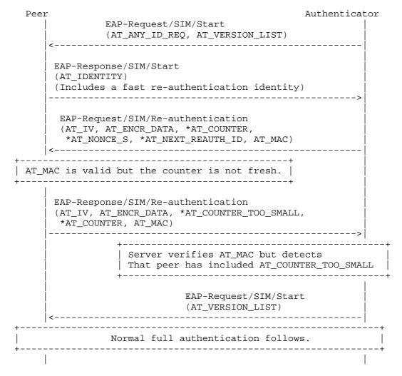
Figure 9: Fast Re-authentication, counter is not fresh
