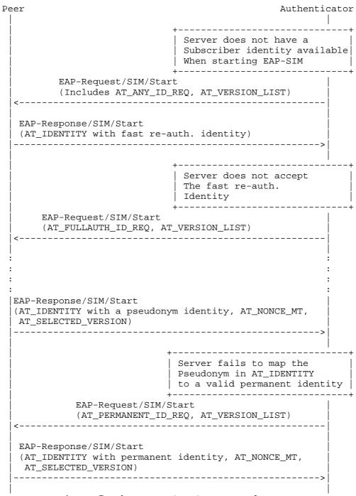
Figure 7: Three EAP-SIM Start rounds
