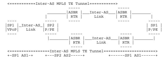
In situations where end-to-end Diffserv paths must be maintained, both SPs' networks may need to provision Diffserv PHB at each hop in order to support a set of traffic classes with compatible performance targets. The subsequent issues regarding Service Level Agreement (SLA) boundaries, reporting and measuring system interoperability and support demarcations are beyond the scope of this document and are not discussed further.
