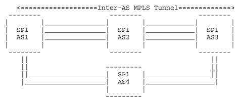
The motivation for inter-AS MPLS TE is even more prominent in a Diffserv-enabled network over which statistical performance targets are to be maintained from any point to any point of the network as illustrated in the diagram below with an inter-AS DS-TE LSP:
