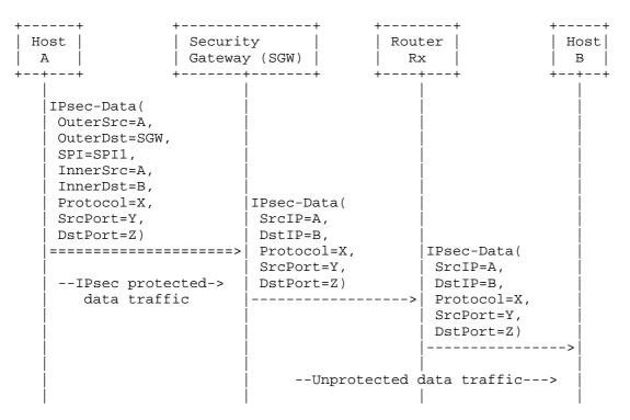
Figure 7: RSVP and IPsec protected data traffic.
