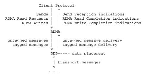
In addition to in-line data flow, read (get()) and update (set()) operations are performed on buffers registered with RDMA as a result of RDMA Read Requests and RDMA Writes, respectively.
