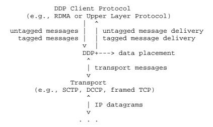
In addition to in-line data flow, the client protocol registers buffers with DDP, and DDP performs buffer update (set()) operations as a result of receiving tagged messages.
