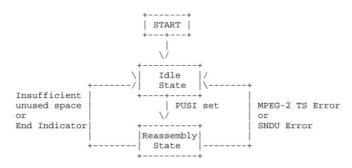
Figure 16: Receiver state transitions
