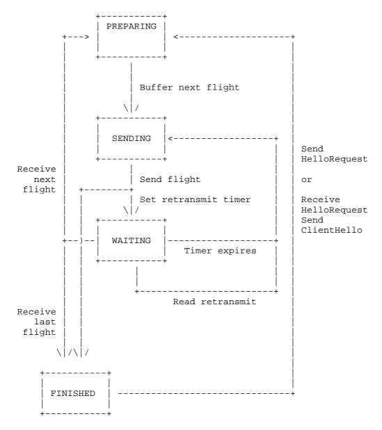
Figure 3. DTLS timeout and retransmission state machine The state machine has three basic states.
