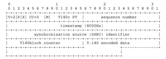
Below is an example of an RTP packet with one redundant T140block using audio/t140c payload format. The primary data block is empty, which is the case when transmitting a packet for the sole purpose of forcing the redundant data to be transmitted in the absence of any new data. Note that since this is the audio/t140c payload format, the redundant block of T.140 data is immediately preceded with a T140block counter.
