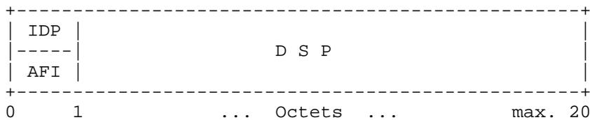
Figure 5 Structure of NSAP Addresses (AFI=0x50 or AFI=0x48)
