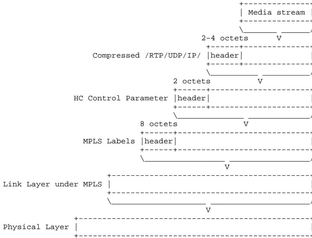
Figure 3: Header Compression over MPLS Media Stream Transport
