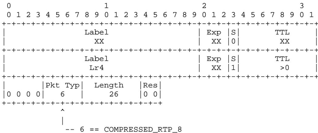
The HC control parameter again changes to reflect another ECRTMP packet type following the control parameter, and shorter length associated with an even more compact encoding of headers. The length field value of 26 comprises:
