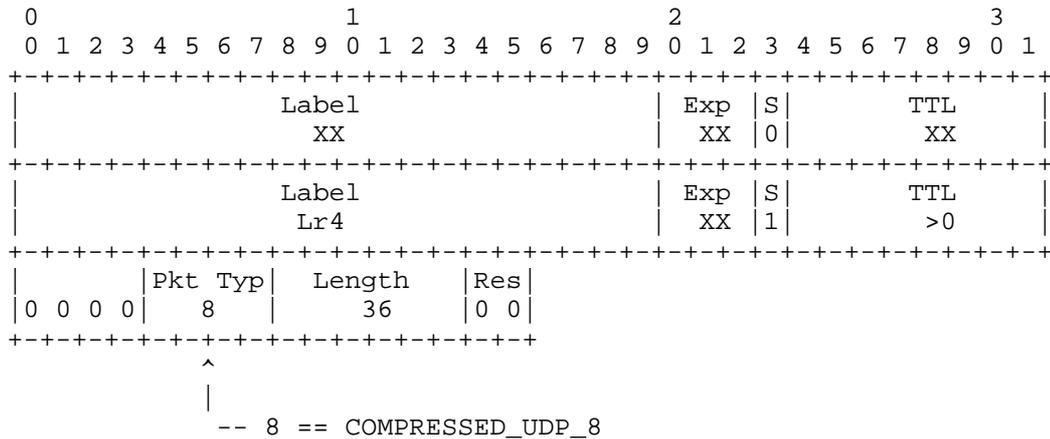
There is no change in the MPLS label stack between the FULL\_HEADER packets and the COMPRESSED\_UDP packets. The HC control parameter changes to reflect another EC RTP packet type following the control parameter, and a change of packet length. The length changes because the new packet type more compactly encodes the headers. The length field value of 36 comprises:
