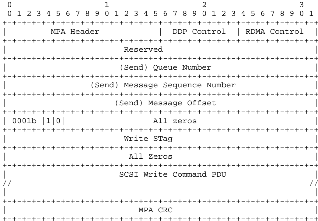
Figure 10. SendSE Message Containing a SCSI Write Command PDU
