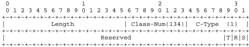
RecoveryPath Transmit Enabled (T): 1 bit
