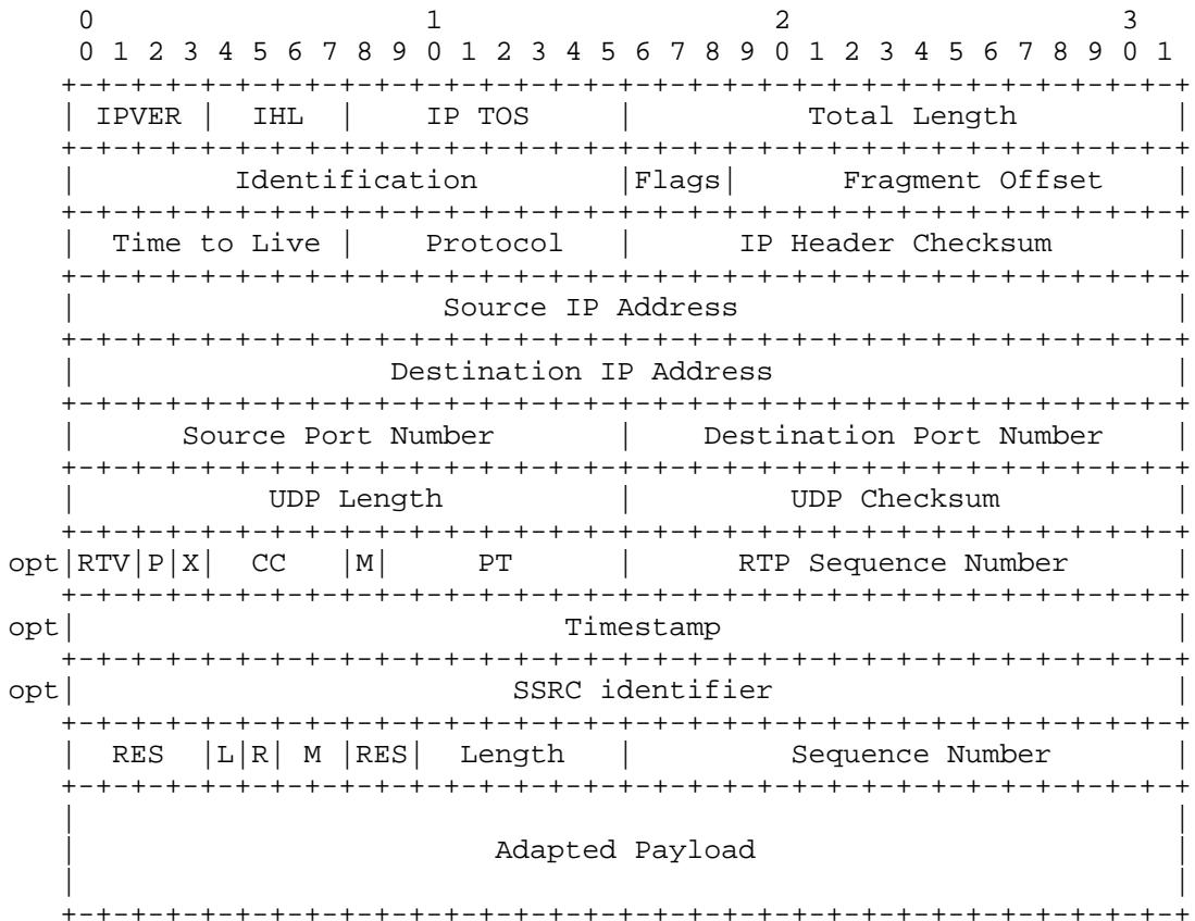
Figure 3. TDMoIP Packet Format for UDP/IP
