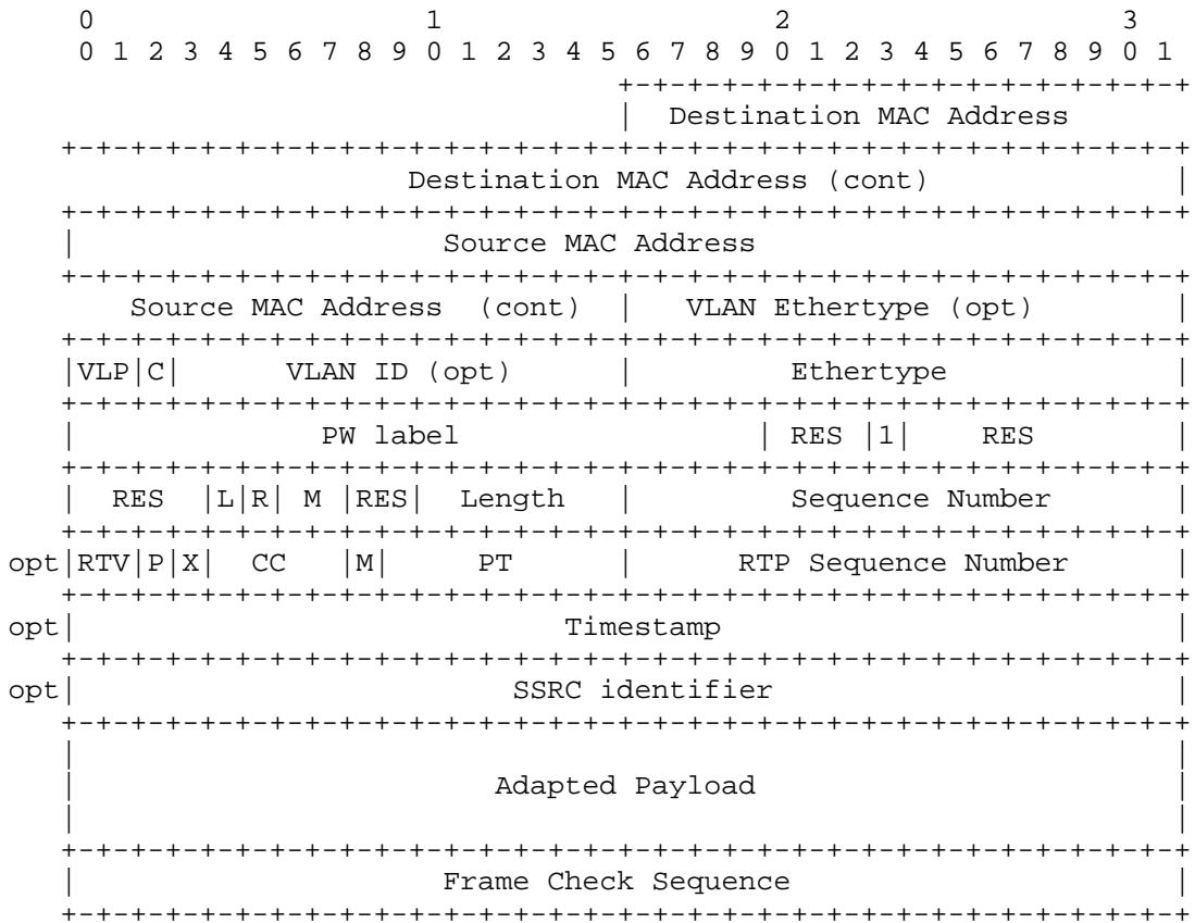
Figure 6. TDMoIP Packet Format for Ethernet
