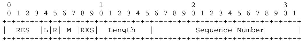
Figure 2. Structure of the TDMoIP Control Word
