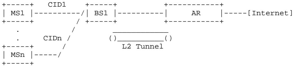
Figure 6: IPv6 AR is separate from the BS
