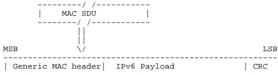
Figure 3: IPv6 encapsulation
