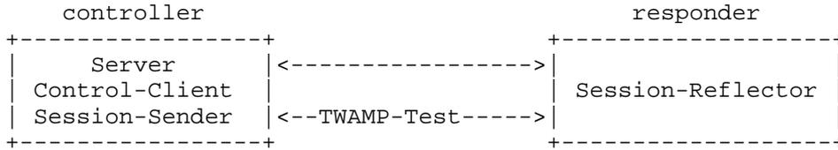
This example provides a simple architecture for responders where their role will be to simply act as light test points in the network. The controller establishes the test session with the Server through non-standard means. After the session is established, the controller transmits test packets to the responder. The responder follows the Session-Reflector behavior of TWAMP as described in section 4.2 with the following exceptions.
