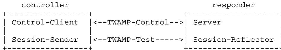
This example provides an architecture that supports the full TWAMP standard. The controller establishes the test session with the responder through the TWAMP-Control protocol. After the session is established, the controller transmits test packets to the responder. The responder follows the Session-Reflector behavior of TWAMP as described in Section 4.2.
