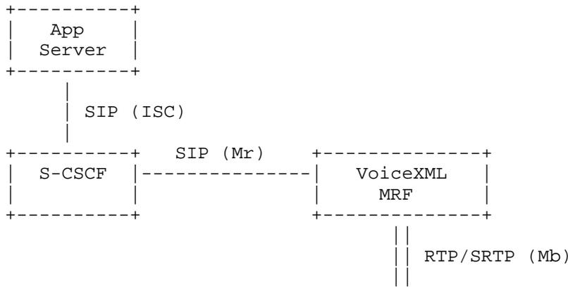
The above diagram is highly simplified and shows a subset of nodes typically involved in MRF interactions. It should be noted that while the MRF will primarily be used by the Application Server via the Serving Call Session Control Function (S-CSCF), it is also possible for calls to be routed directly to the MRF without the involvement of an Application Server.
