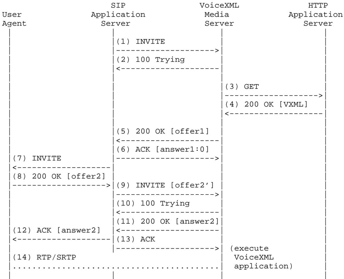
Implementation detail: offer2' is derived from offer2 -- it duplicates the m-lines and a-lines from offer2. However, offer2' differs from offer2 since it must contain the same o-line as used in answer1:0 but with the version number incremented. Also, if offer1 has more m-lines than offer2, then offer2' must be padded with extra (rejected) m-lines.
