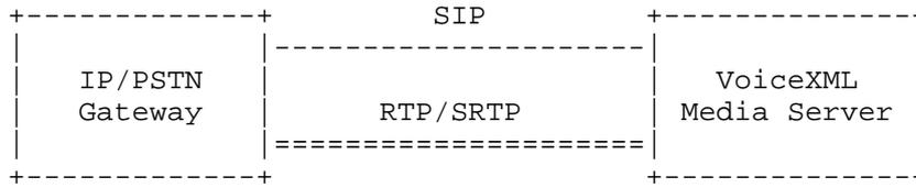
Note also that beyond the invocation and termination of a VoiceXML dialog, the semantics defined for call transfers using REFER are intended to be compatible with standard, existing IP/PSTN (Public Switched Telephone Network) gateways.
