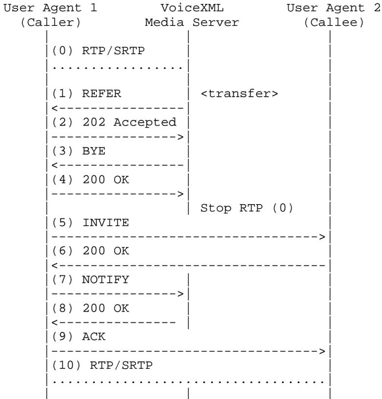
If the `aai` or `aaiexpr` attribute is present on `<transfer>`, it is appended to the Refer-To URI as a parameter named "aai" in the REFER method. Reserved characters are URL-encoded as required for SIP/SIPS URIs [RFC3261]. The mapping of values outside of the ASCII range is platform specific.
