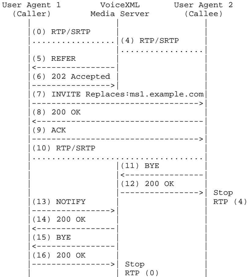
If a response other than 202 Accepted is received in response to the REFER request sent to User Agent 1, the transfer terminates and an error.unsupported.transfer.consultation event is raised. In addition, a BYE is sent to User Agent 2 to terminate the established outbound leg.
