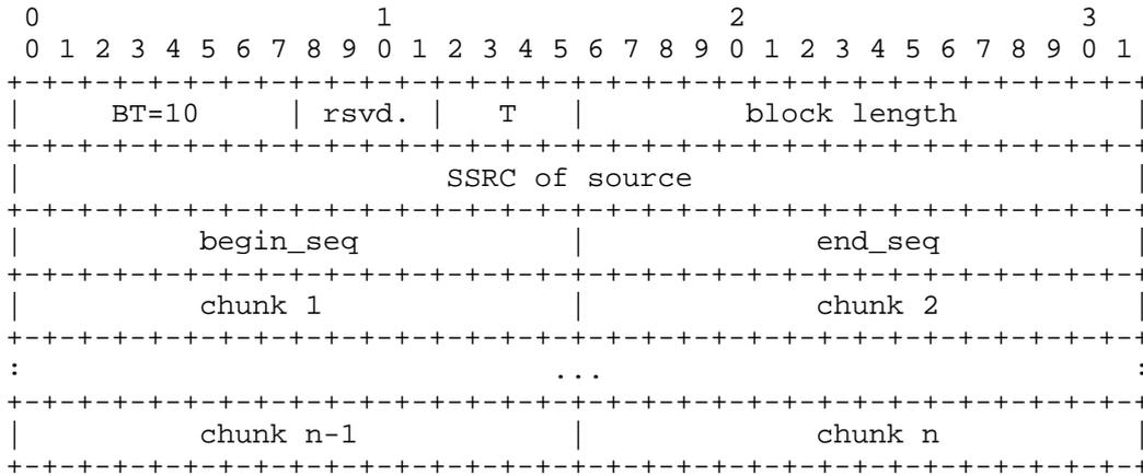
Figure 1: Format for the Post-repair Loss RLE Report Block
