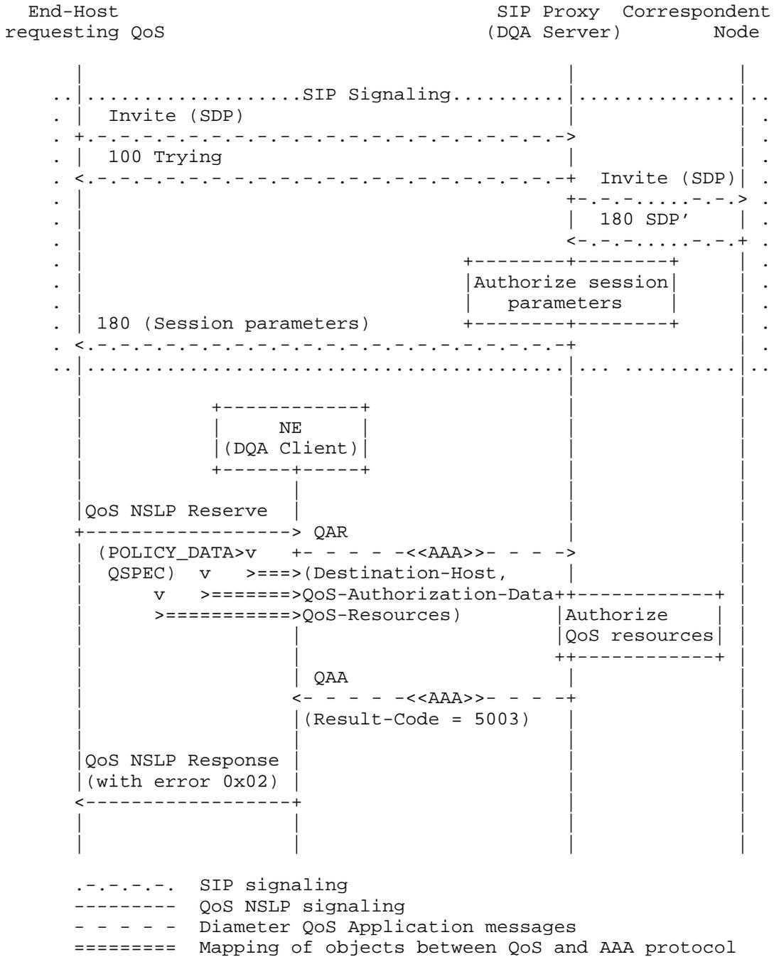
Figure 13: QoS Authorization Example - Pull Mode (Failure Case)
