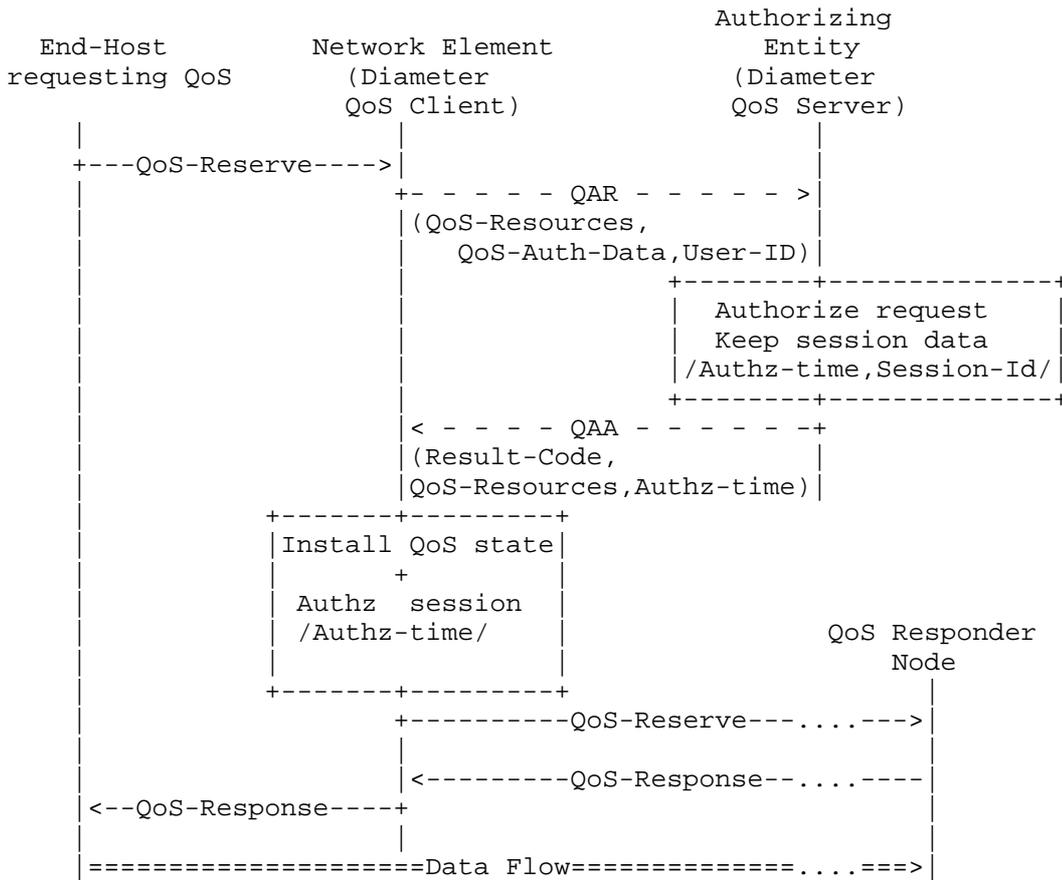
Figure 6: Initial QoS Request Authorization for Pull Mode
