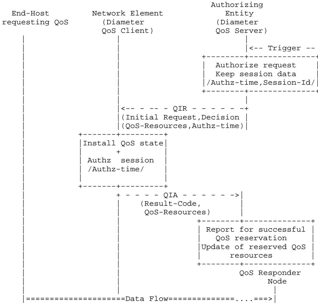
Figure 7: Initial QoS Request Authorization for Push Mode
