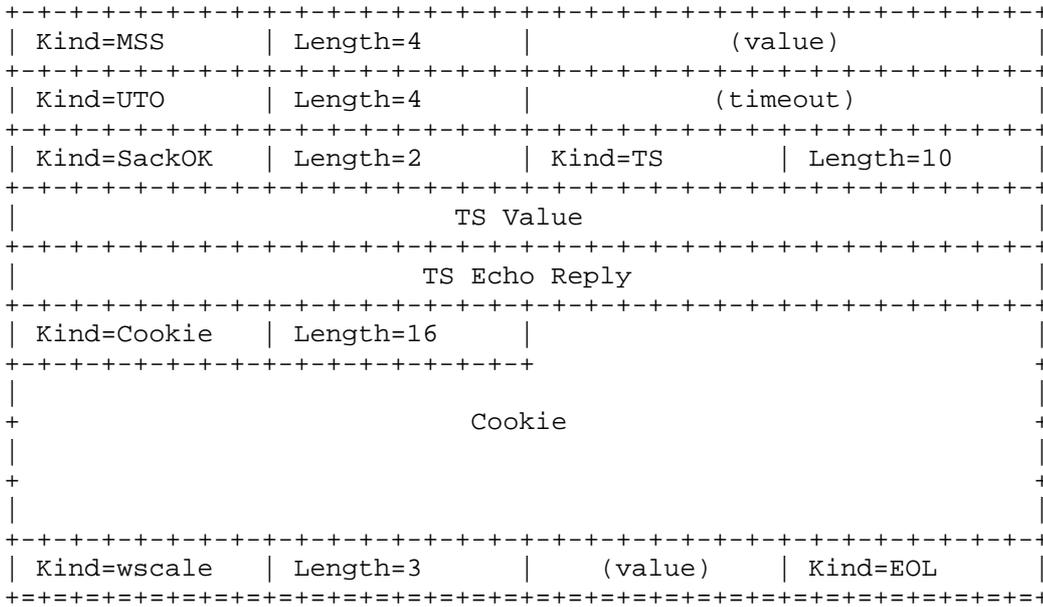
A 14 byte (112-bit) Cookie barely fits with the other recommended options in the maximal 60 byte TCP header (40 bytes of option space).
