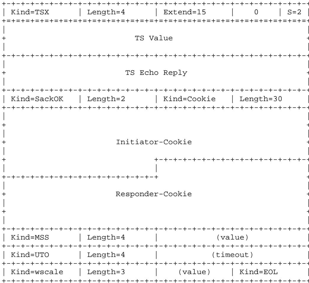
The larger 64-bit (or 128-bit) Timestamps extended option MUST be recognized, although the Responder MAY return a smaller Timestamps extended option.
