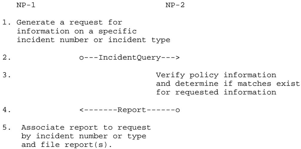
Figure 10. IncidentQuery Communication Flow
