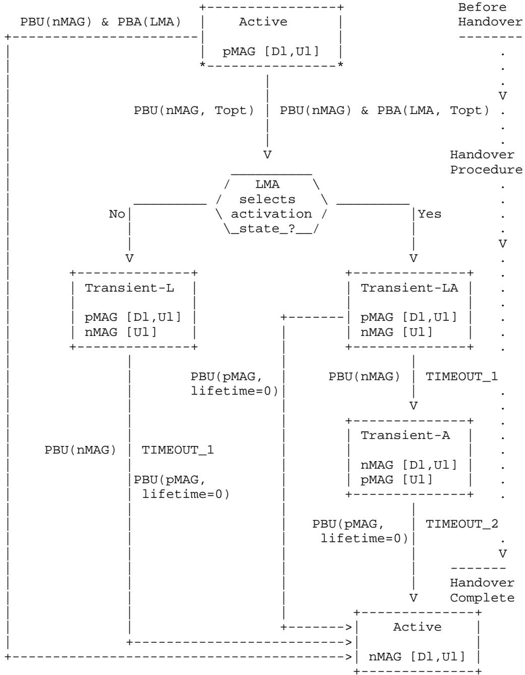
Figure 4: Possible transient forwarding states during a handover
