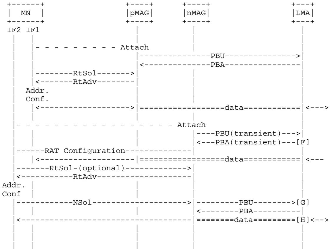
Figure 6: Late path switch with PMIPv6 transient BCEs
