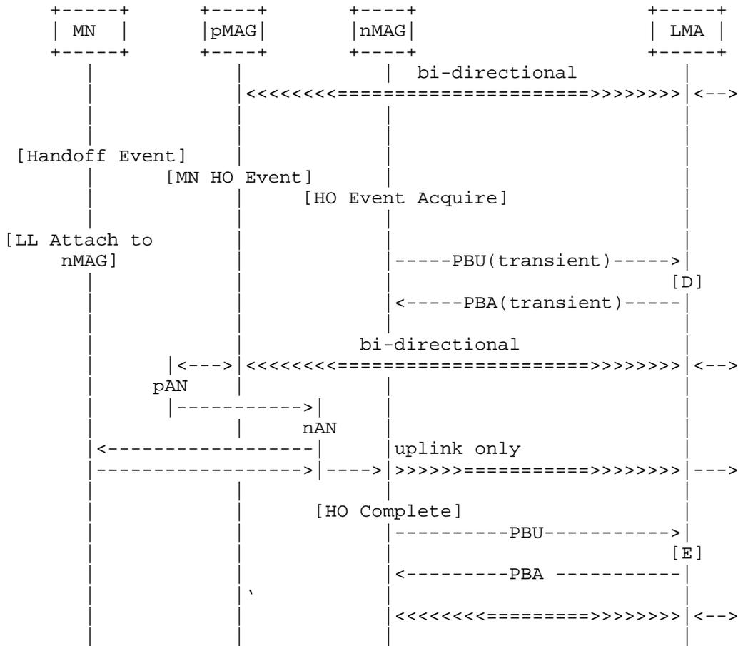
Figure 5: Transient BCE support for an intra-technology handover
